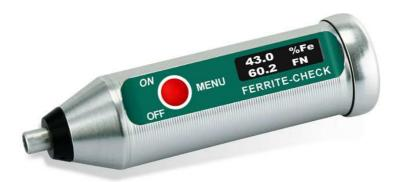
The **List-Magnetik FERRITE-CHECK 110** ferrite content meter is a compact and handy device with an integrated probe for measuring the ferrite content in austenitic and duplex steels according to the Basel standard DIN EN ISO 8249 using the magnetic induction method.
