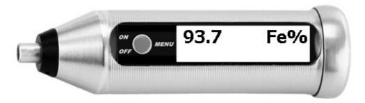
When the measurement type is changed to the average value measurement (**Mode** / **Average measurement**), the current single value and the average value of the measurement series are displayed, since the last time the probe was placed on the object.
