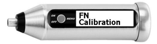
The FN calibration is normally performed on the calibration standard with the lower specified FN value.
