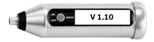
The automatic turnoff time is 2 minutes in the delivery state and can be changed under the menu item **Setup**.
