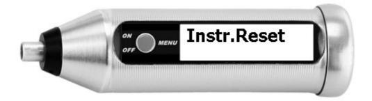
If the device can no longer be calibrated correctly or if any other malfunction occurs, the factory calibration can be reloaded here by performing a device reset. The device switches off automatically.
