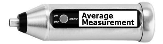
With the average value measurement, measured values are permanently recorded and arithmetically averaged. In this way, you can drag the device over a workpiece and see the current value as well as the average value of all previously measured values. After lifting the probe and placing it on the workpiece again, the average value is reset.
