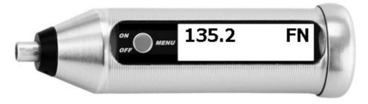
By changing the measuring unit (**Setup** / **Unit**), the measurement can be displayed in Fe%.
