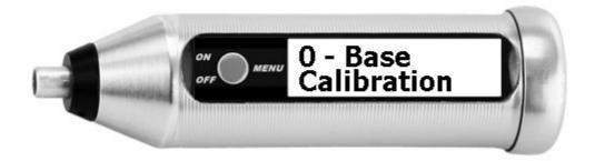
The base calibration is called zero calibration, although its result is not FN 0, but FN 140. FN 140 corresponds to 100% Fe and is the value of full iron or saturated ferrite material.
