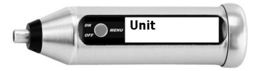
The conversion from FN to Fe% is a simple formula with a constant factor. FN 140 = 100% Fe, the factor is always 1.4.
