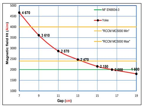
\*The general performance figures provided are indicative as they are specific to each system and may therefore vary slightly. The measurements were taken on a ISO9934-3 C22 metal plate. MPI BATTERY KIT - MAGNETIX MGN3
