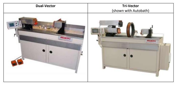
Multi-Vector or Multi-Directional wet horizontal magnetic particle machines can cut inspection time in half by testing for longitudinal and transverse flaws simultaneously. You can test more with less labor and less time which is well suited for production environment.
