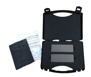
simulate production conditions. Typically one panel is processed using new, unused materials and the other panel is processed using working / in-use materials. Compare the appearance of the panels after processing to assess the performance of the working / in-use materials, noting any degradation from the performance of new, unused materials.
