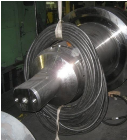
Winding a coil through the part:
