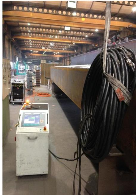
Demagnetization of a steel box girder
