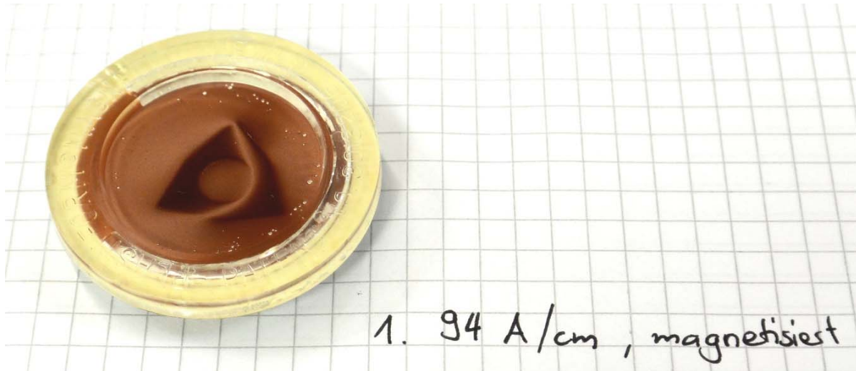
Figure 1: Carbide cutting element seen under the Magnetic Viewer
