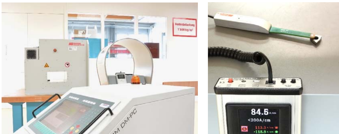
Figure 4: Maurer Magnetic VE-2 Coil Module with 260kA/m, DM-P Power Module and measuring device M-Test LL
