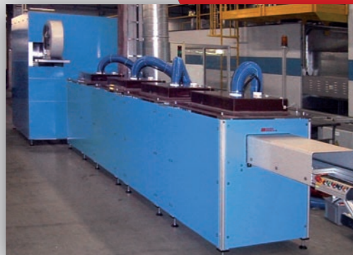
Multiple-stage demagnetization for complex welded structures.
