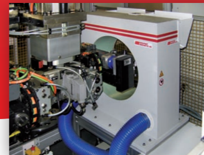
Demagnetization of completely assembled transmission parts for the automotive industry by a powerful degaussing field pulse.
