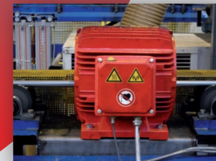
Continuous demagnetization of bars/tubes at transportation speeds of up to 3m/s with the MM RE110 coil.
