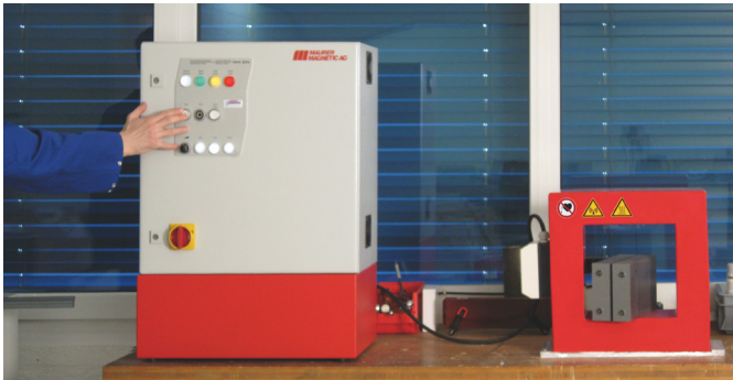
The system is operated at a safe distance to the coil in order to avoid any impermissible field exposure
