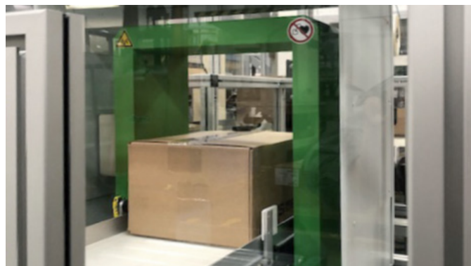
Active demagnetizing pulse for demagnetizing a box with bulk material
