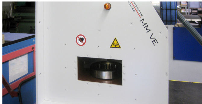
Demagnetizing of assembled roller bearings with pulse technology and high field strength
