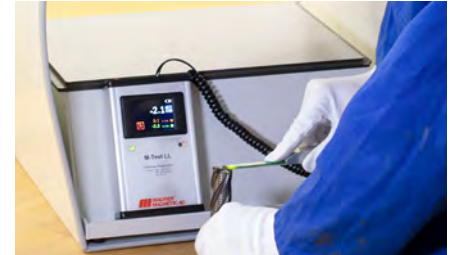
Measurement of residual magnetism of the same cutter in the earth's magnetic field. The induced fields falsify the measurement result from 0.1 \text{ A/cm} to about 2.1 \text{ A/cm}
