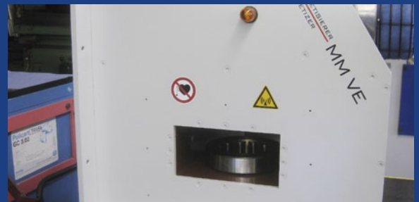
Complete demagnetization of assembled bearings with pulse technology and high field strength.
