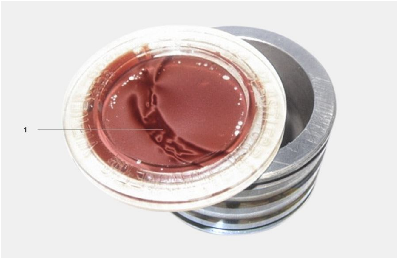
Residual magnetism on ball bearing shell caused by hardening process made visible with the Magnetic Viewer (1)
