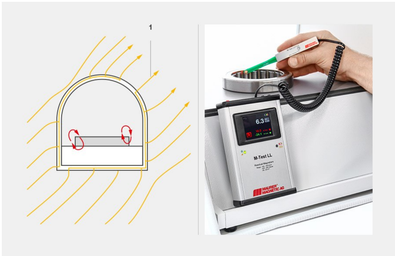
Nearly field-free measuring location: The zero Gauss chamber reliably shields the ambient field (1) and thus enables reproducible residual magnetism measurements.
