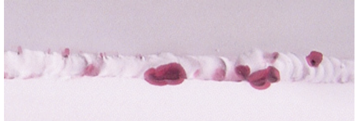
Visible penetrant indications of porosity on weld and stress cracks on metal clamp.
