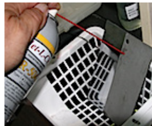
Cleaning Star Burst test panel
