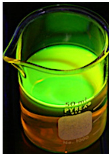
FLP-1 diluted 3 parts water to 1 part penetrant
