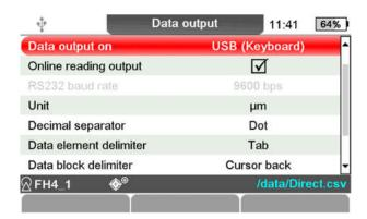
The measured values can now be transferred either individually by pressing the key or directly to the target software if automatic data transfer is activated.
