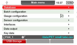
In the main menu, use the "↑" or "↓" keys to select a submenu, e.g. "gauge configuration", and confirm with the "OK" key to access the settings in this submenu.
