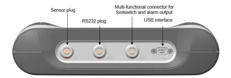
The multifunction socket is used to connect the foot switch or alarm transmitter. The USB socket is used to connect a USB cable to transfer readings or - in connection with the power supply unit - for mains operation and for charging the internal battery.
