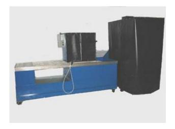
The NDT 1836-WW is a six station system. Each of the tanks measure 18" left to right x 36" front to back x 36" deep. Overall system length is 9', plus 36" wide Inspection Booth.
