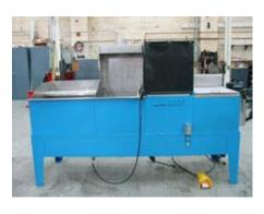
The NDT 1230-PE is an eight station system. Each of the tanks measure 12" left to right x 30" front to back x 16" deep. Overall system length is 9'.
