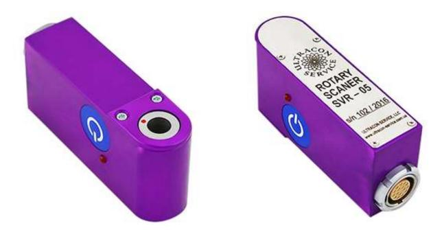
The SRV Rotary Eddy Current Probe Scanner can be used with instruments and probes from GE, Hocking, Rohmannn, Foerster, etc. Rotation speed is variable from (600 to 3000 rpm) and Operating Frequencies from 100kHz to 6MHz. They are primarily used for inspecting bolt holes in airplanes structures and airplane wheel bolt holes, etc. for cracking.
