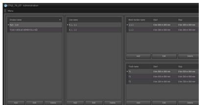
Specialized software of the ETS2-73 flaw detector Program for creation of the track sections to provide the testing and user Administration
