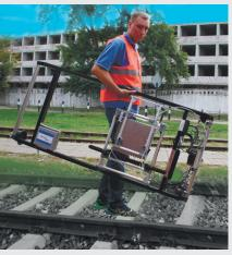
Weight of the assembled flaw detector does not exceed 22 kg. Overall dimensions of the assembled flaw detector are not more than: width - 900 mm; length - 1730 mm; height - 350 mm
