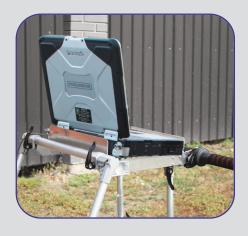
The device allows detecting crosswise and oblique (at 45° to the longitudinal axis of rail) surface cracks of operational origin.
