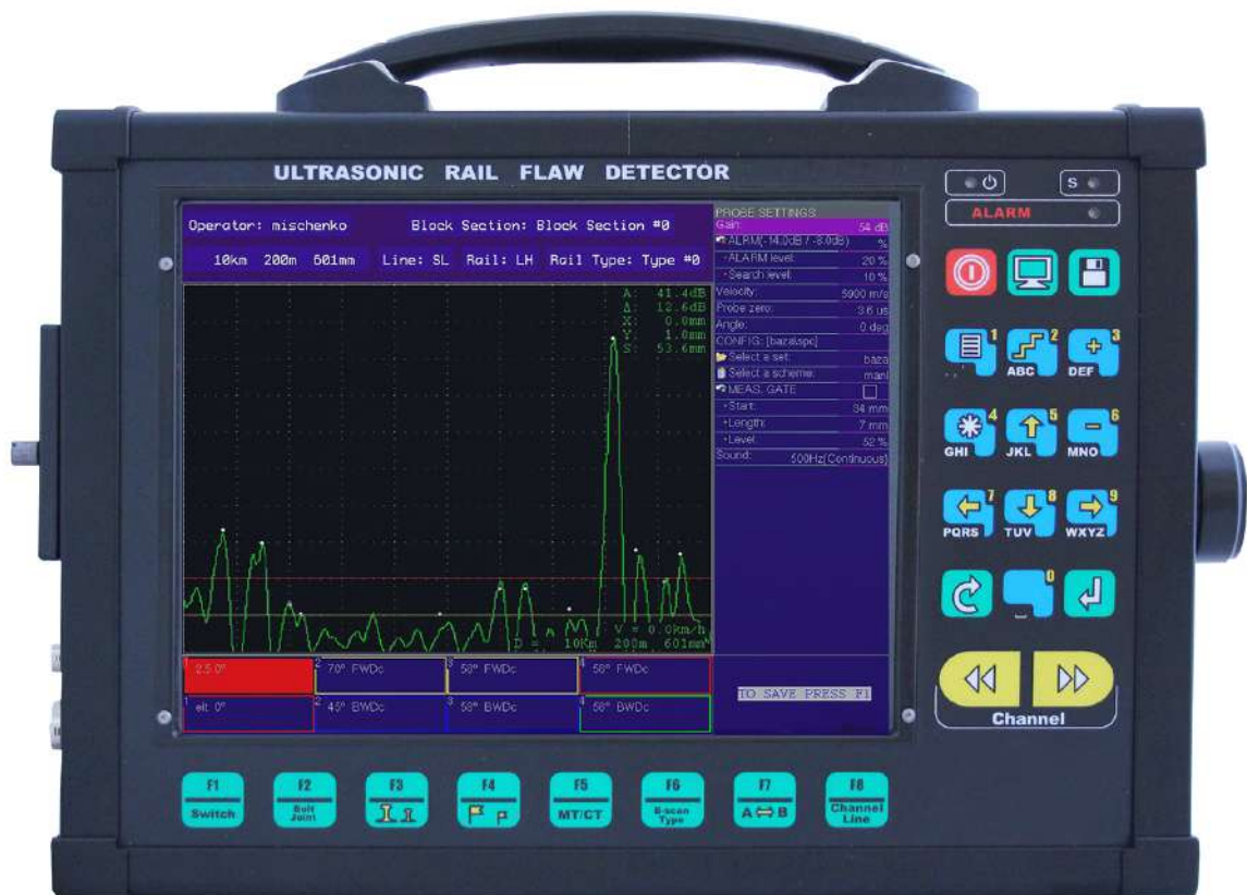
Figure 7 – Appearance of the electronic unit of the ultrasonic flaw detector
