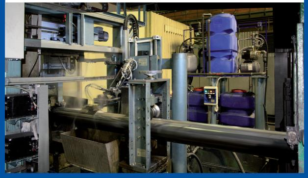
Conventional ultrasonic inspection in FD System is performed using 45-degree and/or 70 degree UT probes. 45-degree probes are sensitive to surface-breaking ID/OD cracks. The 70-degree probes are sensitive to mid-material flaws.
