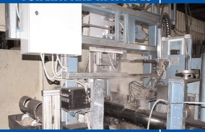
Monitoring of the ERW weld quality in in-line welding area Real Time Presentation of Wall Thickness Data, in engineering units, on the tube mill
