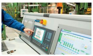
**HIGH LEVEL MAN-MACHINE INTERFACE** Extremely hard environment conditions are applied by IP64 OKO-22M-UT electronic units Fast Software provides high-speed tube testing with up to 12 channels simultaneously.
