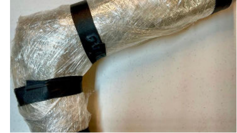
PiX Pikena Imaging Sample Oil & Gas (Corrosion under Insulation)
