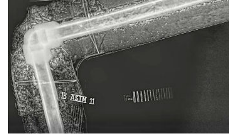
PiX Pikena Imaging Sample Oil & Gas (Corrosion under Insulation)
