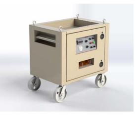
Line Voltage & Current Requirements with Standard 12V Secondary Output VAC: 240, 60Hz, Recommended Service Size: 150, Fuse Type: 150 Time Delayed Recommended Wire Size: 1 AWG For s100 Ft. of Run VAC: 480, 60Hz, Recommended Service Size: 75, Fuse Type: 75 Time Delayed Recommended Wire Size: 4 AWG For s100 Ft. of Run
