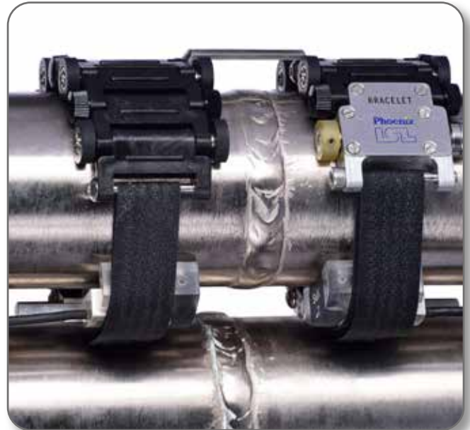
Dual Bracelet configuration scanning double sided phased array on 2" pipe
