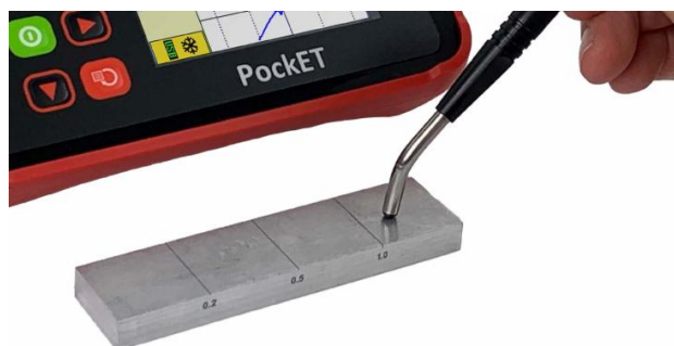
200kHz – ATBA Aluminum Test Block, 0.2, 0.5, 1.0mm slots
