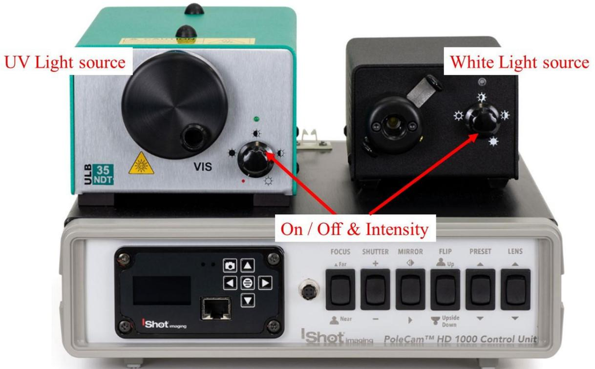
Figure 3 ON/Off Controls Light Sources
