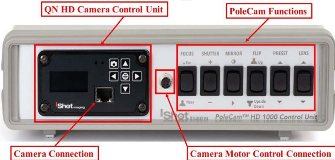
Figure 1 Control Unit Connections & Controls Front
