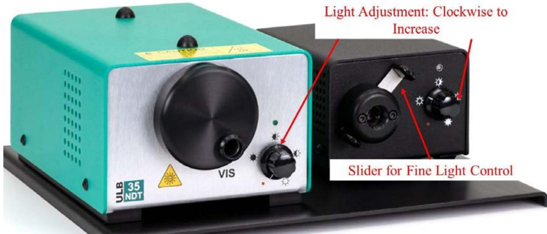
Figure 6 Light Source Controls
