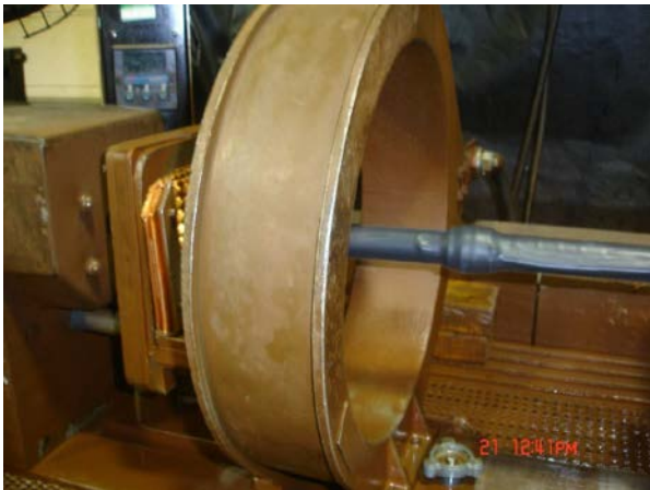
Mag unit coil is too far to the left of transducer coil.
