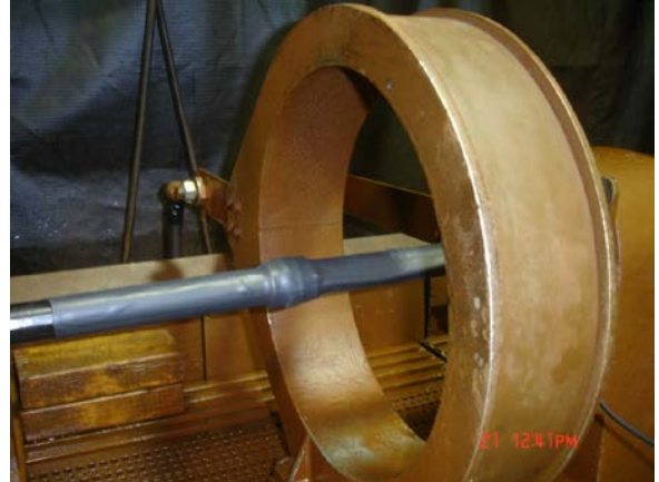
Mag coil too far to the right of the transducer coil.
