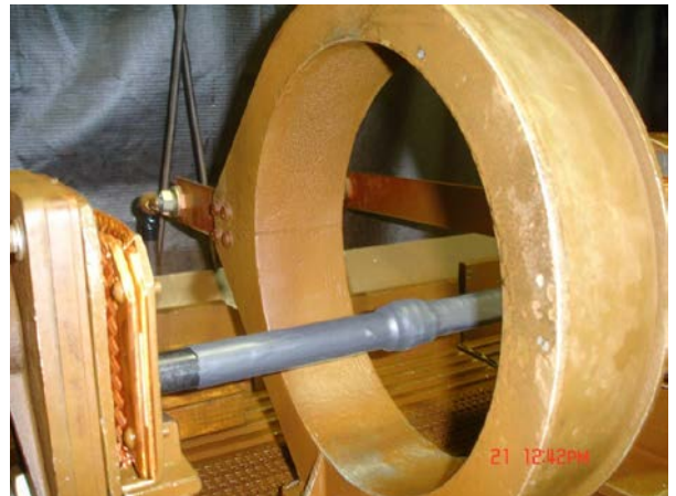
Transducer is clamped too low in the headstock/tailstock, raise it up until it is in the center of mag unit coil.
