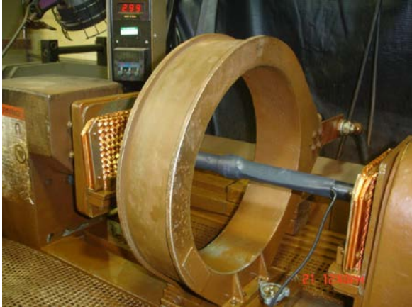
CORRECT – Transducer is well centered coaxially and coplanarly in the mag unit coil.
