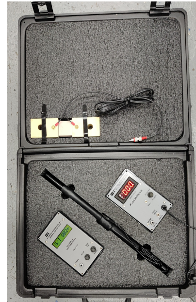
Test kit ammeter, shot timer and quick break tester
