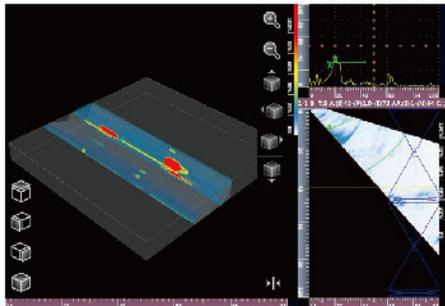
PA 3D: Supports 3D display of workpiece, probe, wedge, beam simulation and flaws.
