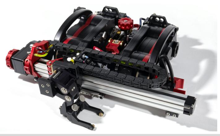
**ScanTech utilizes our STC distributed, modular control system.** This communication architecture minimizes conductors making the umbilical significantly lighter. It also offers easy expandability for an additional axis or add-on features, making this a very versatile platform for your scanning requirements. The Apex will easily adapt to nearly any application.
