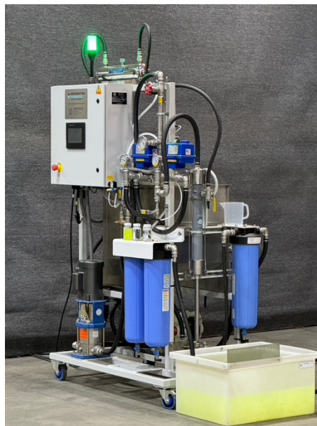
EUS-E – FPI Wastewater Filtration System
