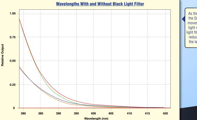
As the wavelength of the QUADRAN<sup>™</sup> 365 moves into the visible light range, the black light filters significantly reduce the output of the lamp at 400 nm. The QUADRAN™ 365 can be quickly mounted for in-line inspections using various Spectroline<sup>®</sup> accessories (FA-100 flexible arm shown).
