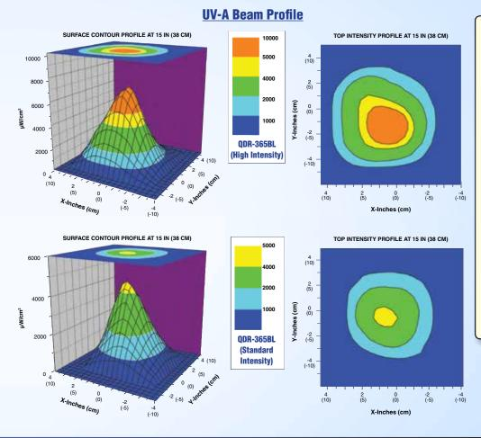
The **QDR-365BL** is equipped with a faceplate with <u>integral black</u> <u>light</u> filters that reduce the output of wavelengths longer than 400 nm. When in the *high intensity* mode, the lamp provides a nominal steady-state UV-A intensity of 7,000  $\mu$ W/cm<sup>2</sup> at 15 inches (38 cm).
