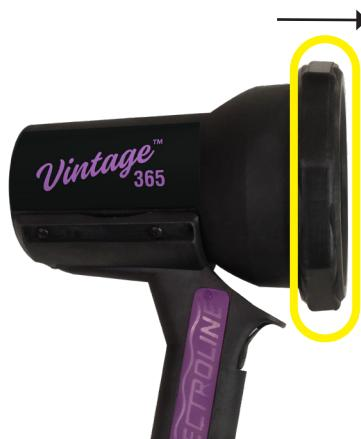
The glass filter will remain inside the protector. To remove the glass filter, peel around the edge of the rubber cover/filter holder and push the glass filter out. To replace or reinsert the glass filter into the rubber cover/filter holder, slide the glass filter into the channel of the rubber cover/filter holder. Manipulate the rubber cover around the filter. Ensure the glass filter is evenly seated.
