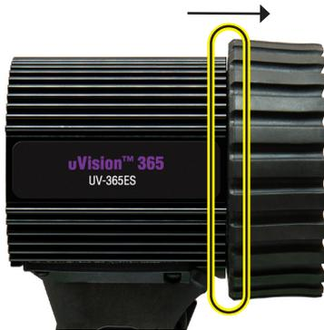
The Clear Borofloat Filter will remain inside the protector. To remove the Clear Borofloat Filter (130089), peel around the edge of the rubber cover/filter holder and push the filter out. To replace or reinsert the Clear Borofloat Filter into the rubber cover/filter holder, slide the Clear Borofloat Filter into the channel of the rubber cover/filter holder. Manipulate the rubber cover around the filter. Assure the filter is evenly seated.
