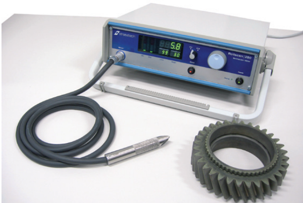
Manual Barkhausen Noise measuring with Rollscan 250
