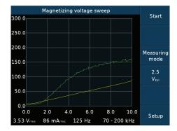
Magnetizing voltage sweep show saturizing of the Barkhausen Noise signal helping to optimize the magnetizing for measurement.
