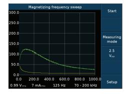
Magnetizing frequency sweep shows the frequency, with which the Barkhausen Noise signal is highest and thus the resolution of Barkhausen Noise best for finding defects.
