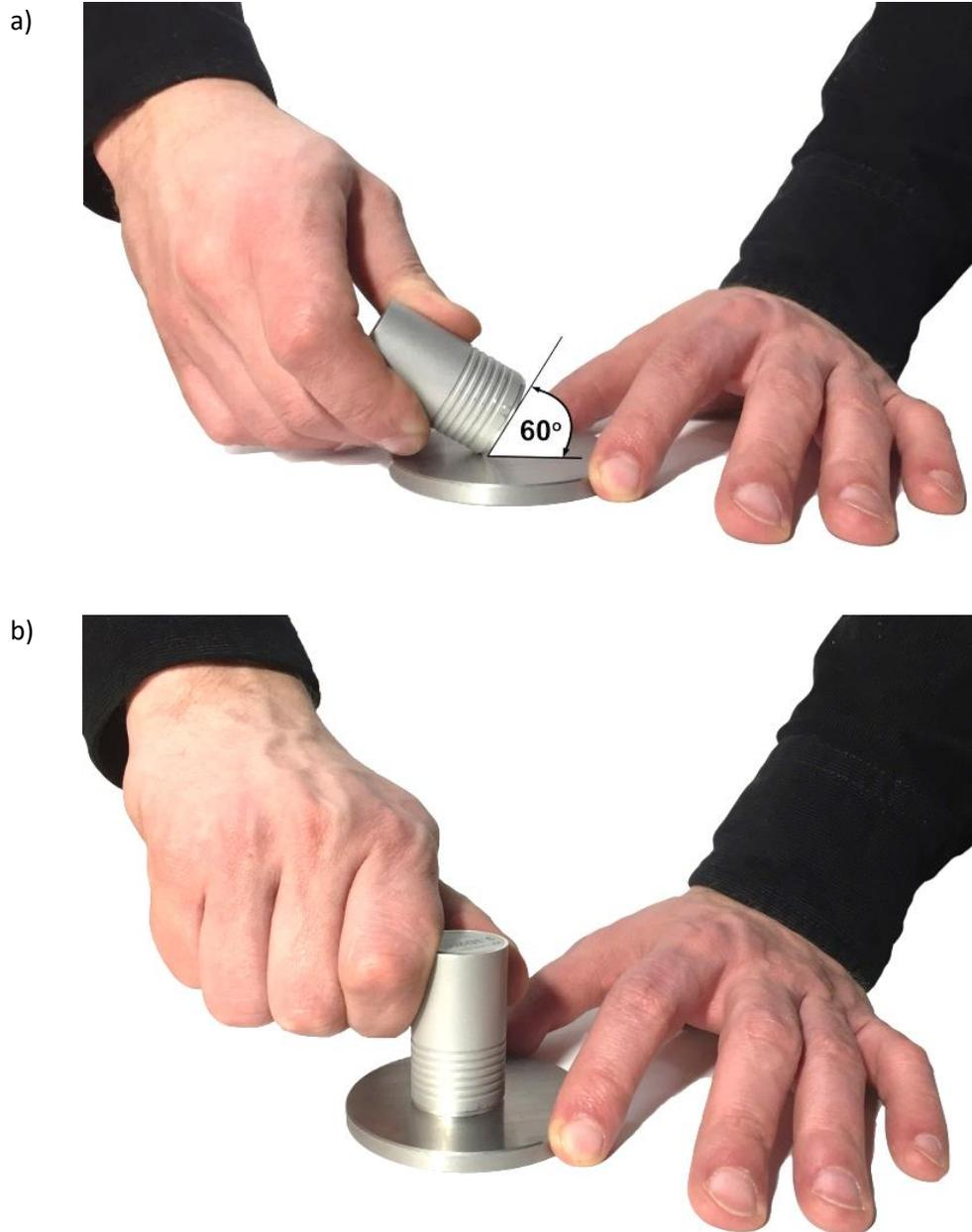
Figure 1.2 – Installation of EMA transducer
