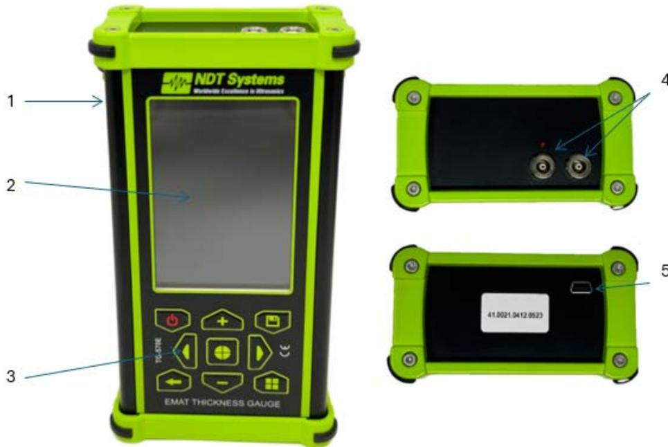
1 – Case; 2 – Contrast Color LCD/TFT Display; 3 – Keyboard; 4 – Transducer Lemo-00 Ports; 5 –Mini-USB Slot.
