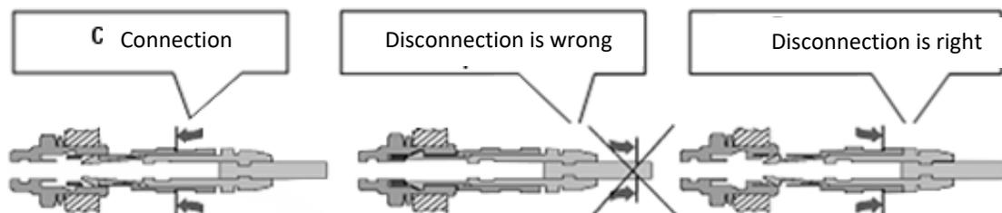
Figure 2.2 – Handling of the connectors
