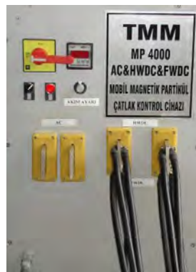
Figure 3. Control Panel (sample)
