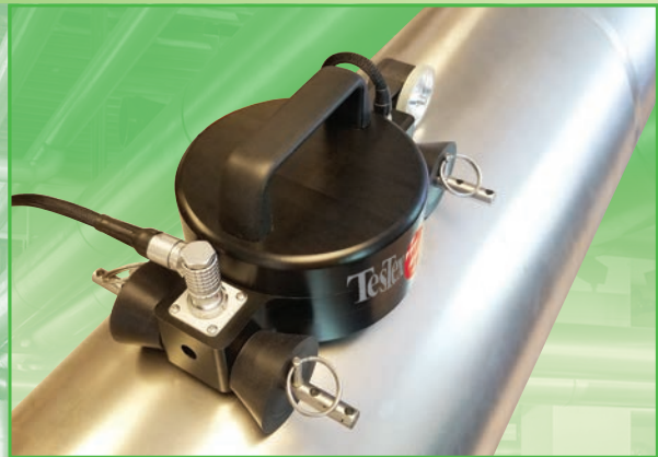
OSET Scanner Performing a Linear Scan
