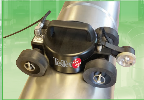
OSET Scanner Performing a Circumferential Overlap Scan
