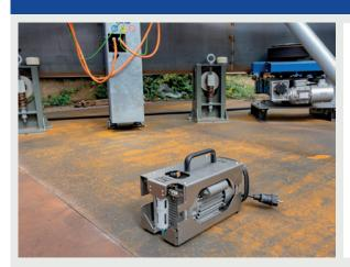
We offer an ultra high-performance dry vacuum pump (8m³/h - 150 mbar vacuum) in 220V, perfectly suited for the most demanding field conditions, with optimal reliability and minimal maintenance.
