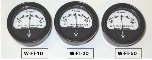
A magnetic field of under 10 Gauss is typically not strong enough for Magnetic Particle Inspection (MPI), thus the W-FI-10 is used to ensure a workpiece is demagnetized. A magnetic field, for MPI, should be approximately 18 to 24 Gauss, thus an inspector uses the W-FI-20 to ensure his field is strong enough. A workpiece can be magnetically saturated prior to or after inspection, and these strong fields are evaluated with a W-FI-50.
