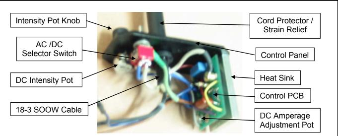
The WE-7 has had several series of Printed Circuit Boards manufactured for use with this model. While function of the PCB has remained the same, the design, component selection, and physical mounting has changed. If an older series of PCB is to be changed, it is recommended that the Heat Sink also be changed. The mounting of the Heat Sink to the Control Panel has remained unchanged.
