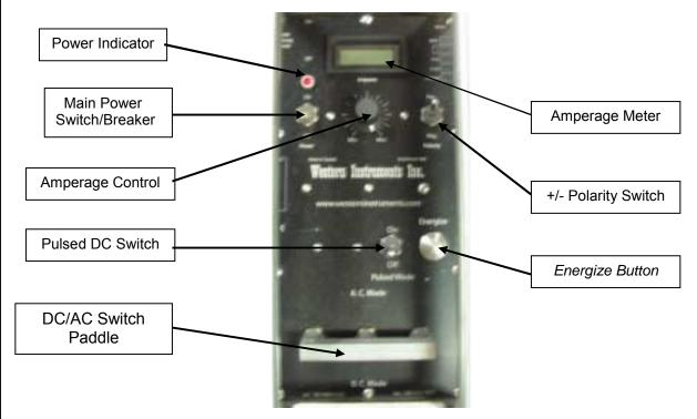
**DC/AC Switch Paddle** The dual position paddle is 3 standard switches 'ganged' together, to allow operators to select either DC Mode (normal operation) or AC Mode. For DC operation the paddle is in the down position (as shown),and is placed in the up position for AC Operation.
