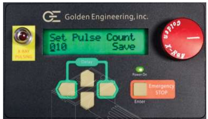
Use LEFT / RIGHT arrow to select Digit Use UP / DOWN arrows to change number Pulse setting from 001 to 999*
