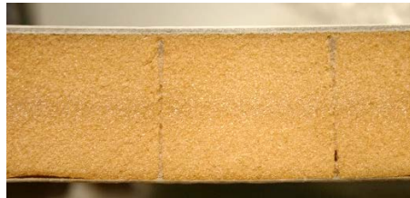
Glass fiber skins with wood core
