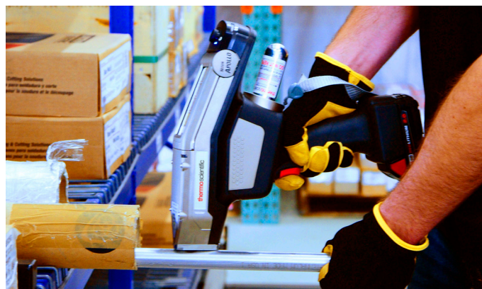
The Niton Apollo in use, validating a Mill Test Report (MTR) prior to fabrication.
