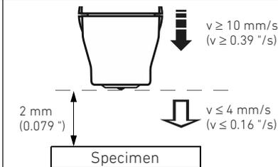
Lift-off distance between 2 measurements  $\geq 10 \text{ mm}$  ( $\geq 0.32''$ )
