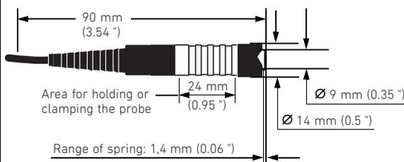
Probe cable length: 1.5 m (59.06"), other cable lengths on request<sup>1</sup>
